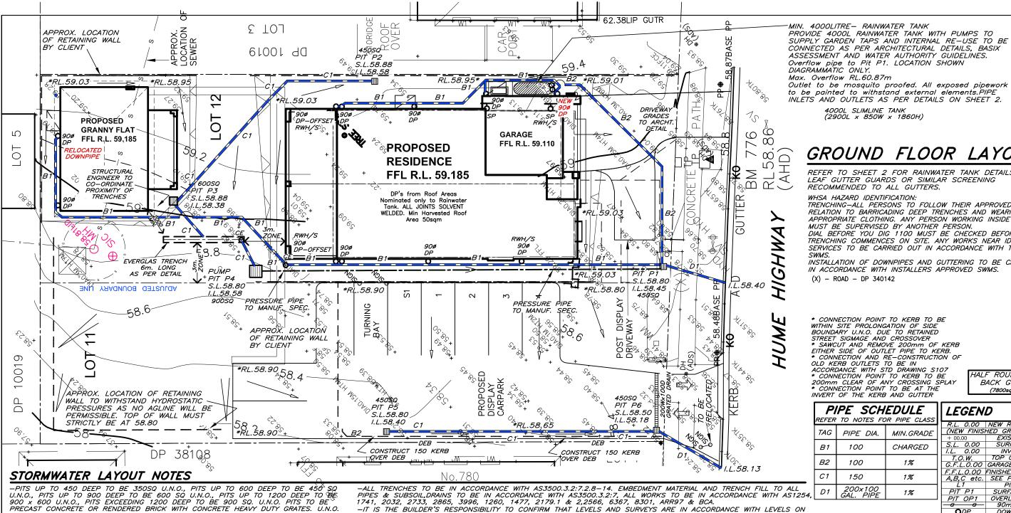
LIGHT DUTY PITS AND GRATES MAY BE USED ONLY IN LIGHT/FOOT TRAFFICABLE AREAS. U.N.O. ALL PITS TO BE BENCHED TO DISCHARGE PIPES U.N.O. GAL. STEP IRONS TO ALL PITS EXCEEDING 900 DEPTH.
